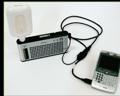
Toshiba Dynario charger (fuel cell) and methanol cartridge.
